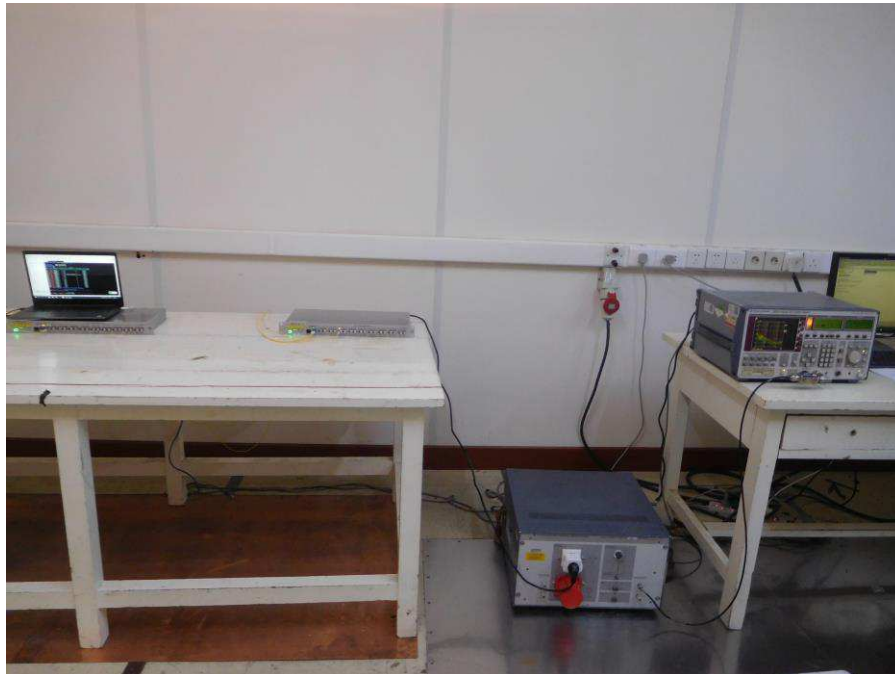
Photograph 2: Set-up for measurement of radiated emission
